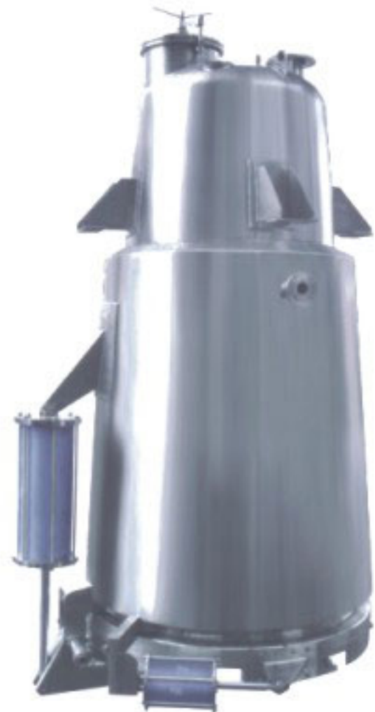
倒锥型提取罐 Upside-sown taper type extracting tank
